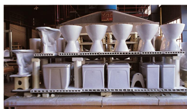
NSiC beams applied in shuttle kiln of sanitary ware
